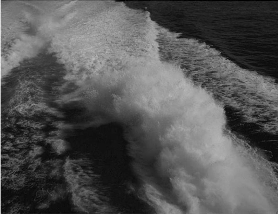
FIGURE 7. A 'rooster tail' generated by a Seacat. The lower right of the photograph is where the highly turbulent propulsive jet has just come out from beneath a hull.
